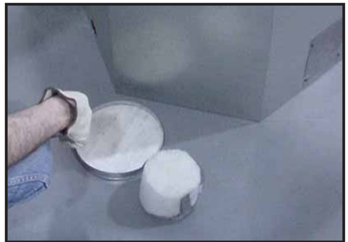
Figure 6.11 Discard the seal cap, remove and discard the insulation basket.
