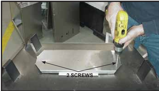
Figure 6.1 For top vent, remove the two screws holding the top heat shield in place.
