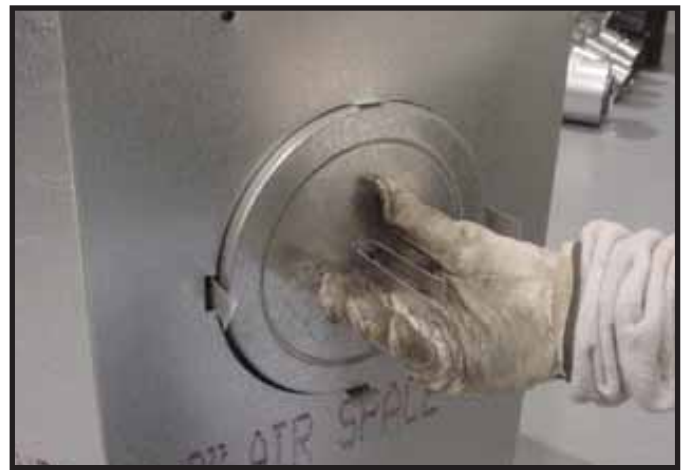
Figure 6.10 Fold the center parts of the retaining band out and use to remove the seal cap.
