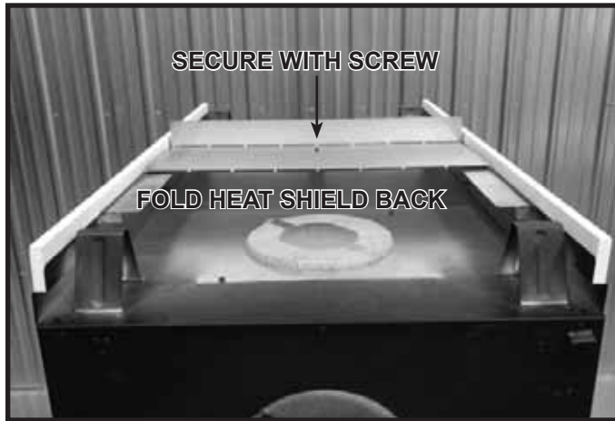
Figure 6.2 ST-36TR-IFT Only: Fold heat shield back and secure with screw.
