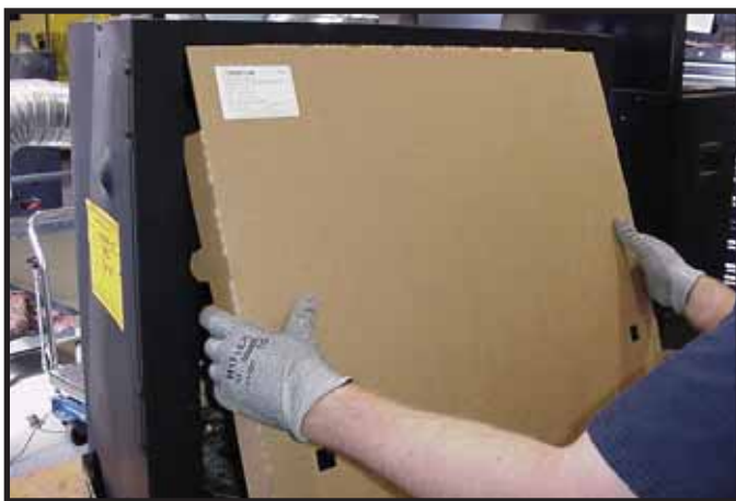
Figure 11.5 Installation of Splatter Guard
