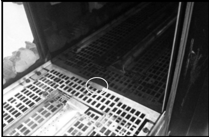
Figure 10.8 Position Glass Clip and Install Glass Panel
