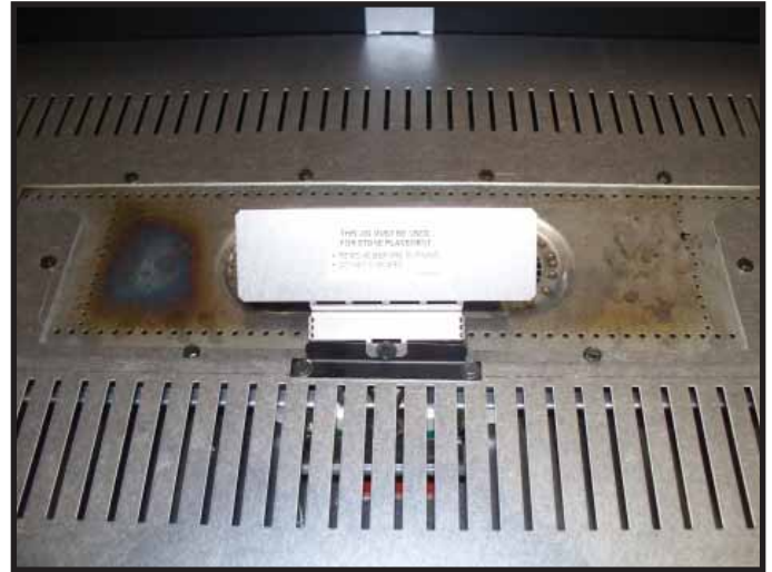
Figure 14.5 Rock Fixture Assembly Installed
