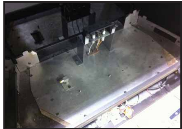
Figure 11.2. Remove Valve Plate Screws
