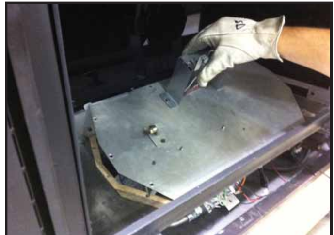
Figure 11.3. Remove Valve Plate
