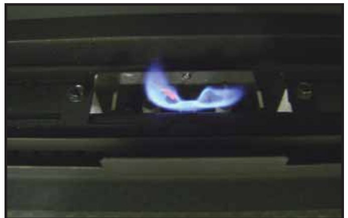
Figure 3.1 IPI Pilot Flame Pattern
