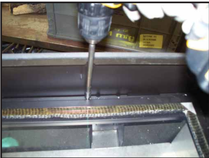
Figure 9.4. Gas and Electrical Access - Remove Glass Window
