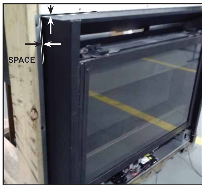
Figure 11.15 Splatter Guard Installation
